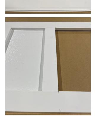
Turn the screen over and mark and fix the mid-bar length into position as you did previously
