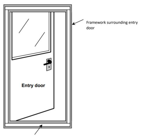
Build off frame around your door frame including the bottom if appropriate
