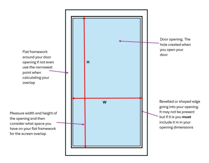
Measure the width and height of the opening including any bevelled edge on the door frame going into the opening and add 40mm to each measurement. This will give you a 20mm overlap on the door frame either side (i.e. half the width of the screen frame).
